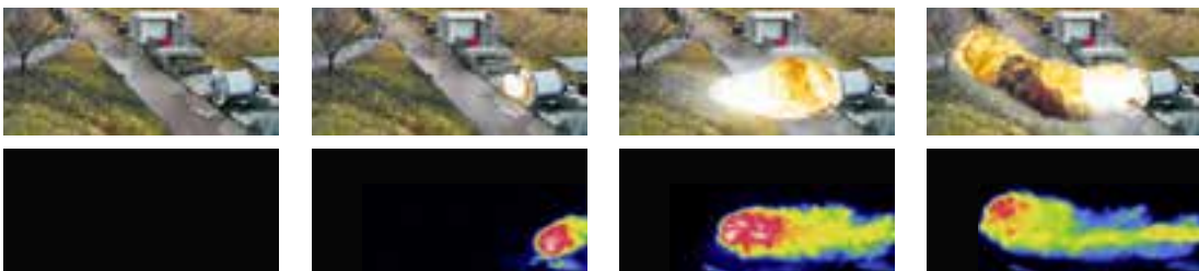
Thermographic investigation of a dust explosion: conventional explosion venting with an explosion vent.
